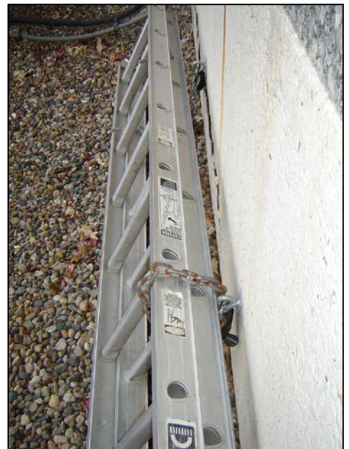
The photo above demonstrates how to properly store a ladder outside the building using a good quality lock and chain that is securely attached to the building's concrete foundation.
