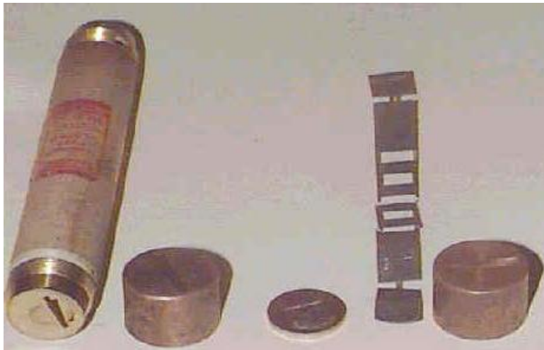
This image shows a renewable fuse and its components. The element is inserted into slots on the top and bottom of the fuse, and the threaded caps screw on and apply pressure to the element. (Photo courtesy of Hartford Steam Boiler)
