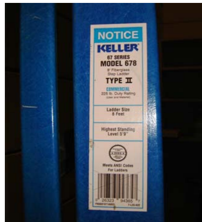
This photo is an example of a rating label that is affixed to a fiberglass step-ladder. This particular ladder is a type II.
